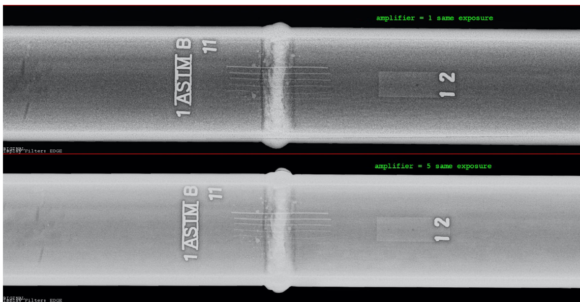
Figure 6: Comparison of adjustments in the amplifier setting for the HPX-DR 4336 DDA. Even though the pixel intensities are also virtually the same, the image quality for the image on the bottom is significantly better from White, B., Presentation “Exposure Guidance and the Myth of Pixel Value Dependence for Digital Detector Array Radiography” ASNT Annual Conference, Virtual, 2020. [8]
