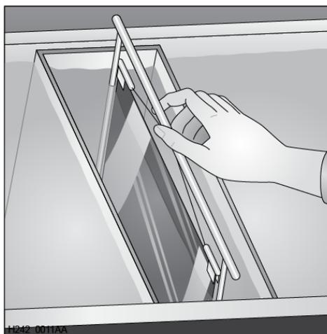
If facilities permit, use a final rinse with a rinsing (wetting) agent to speed drying and prevent water marks. Immerse film for about 30 seconds, and then drain for several seconds.
