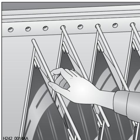
Dry the film at room temperature in a dust-free area or suitable drying cabinet. The temperature must not exceed 49 °C (120 °F). When the film is dry, remove from hangers and insert into envelopes.
