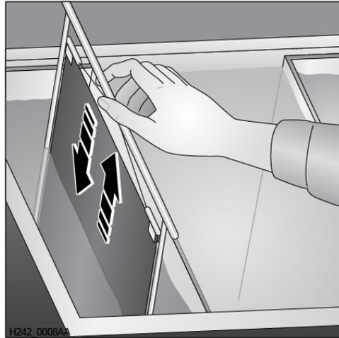
Immediately after immersion in the developer, tap the hanger to dislodge air bubbles. Do not agitate further.
