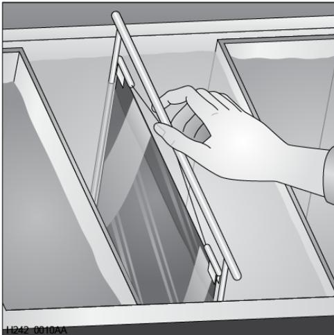
When the timer ends, place the film in the stop bath for 30 seconds. Agitating moderately, lift from the stop bath and drain well.
