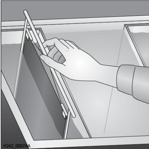
To avoid streaking, completely immerse the film smoothly and without pausing. Start the timer.
