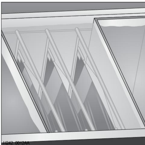
Place the film hangers in a tank of running water for **10-30 minutes**. Keep ample space between the hangers (water must flow over the top).
