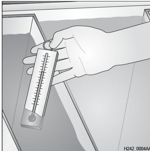
Check the temperature of the solutions with an accurate thermometer, rinsing it off after checking each one. Adjust the temperature as needed.
