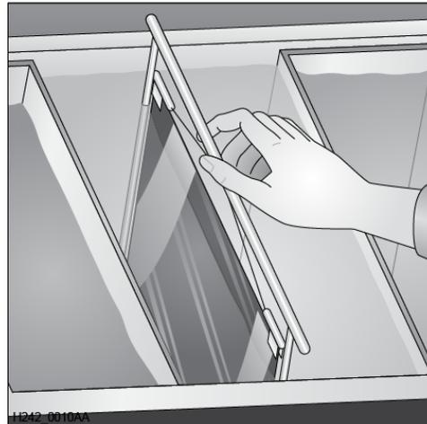
Immerse the film in the fixer for **3-6 minutes**, agitating for **5 seconds every 30 seconds**. Film should remain in fixer for twice the time it takes to "clear" it (when the milky look disappears). **Never fix film for less than 3 minutes.**
