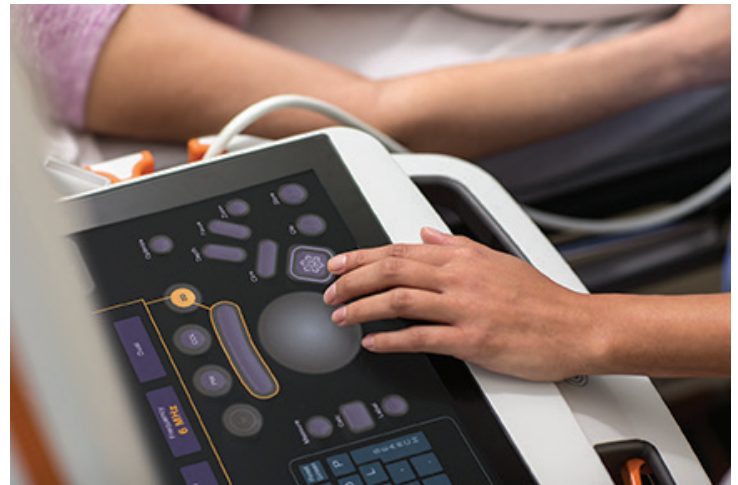
Figure 3: Textured controls help sonographers distinguish between keys quickly and intuitively.
