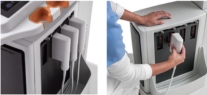
Figures 6 & 7: Multiple transducer ports reduce the need to change transducers by plugging them in. When necessary to change the transducer, this should be easy to accomplish using one hand.
