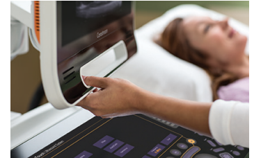
Figures 4 & 5: A handle allows the sonographer to easily reposition the monitor with one hand.
