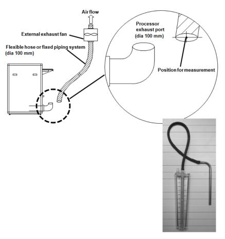
NOTE: If the ventilation tubing is connected to house-internal exhaust system, an air-gap of 5 cm (2 in.) must be provided accordingly.
