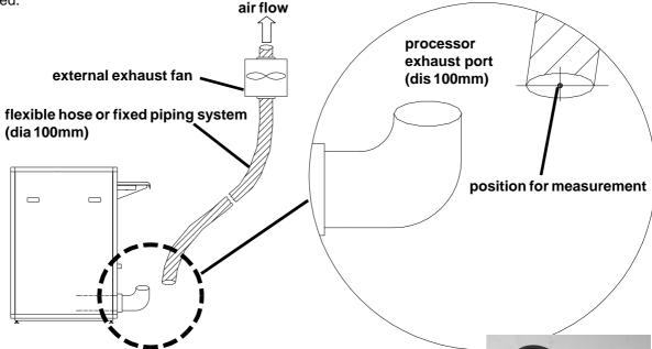
NOTE: If the ventilation tubing is connected to house-internal exhaust system, an air-gab of 5cm (2 inch) has to be provided accordingly.
