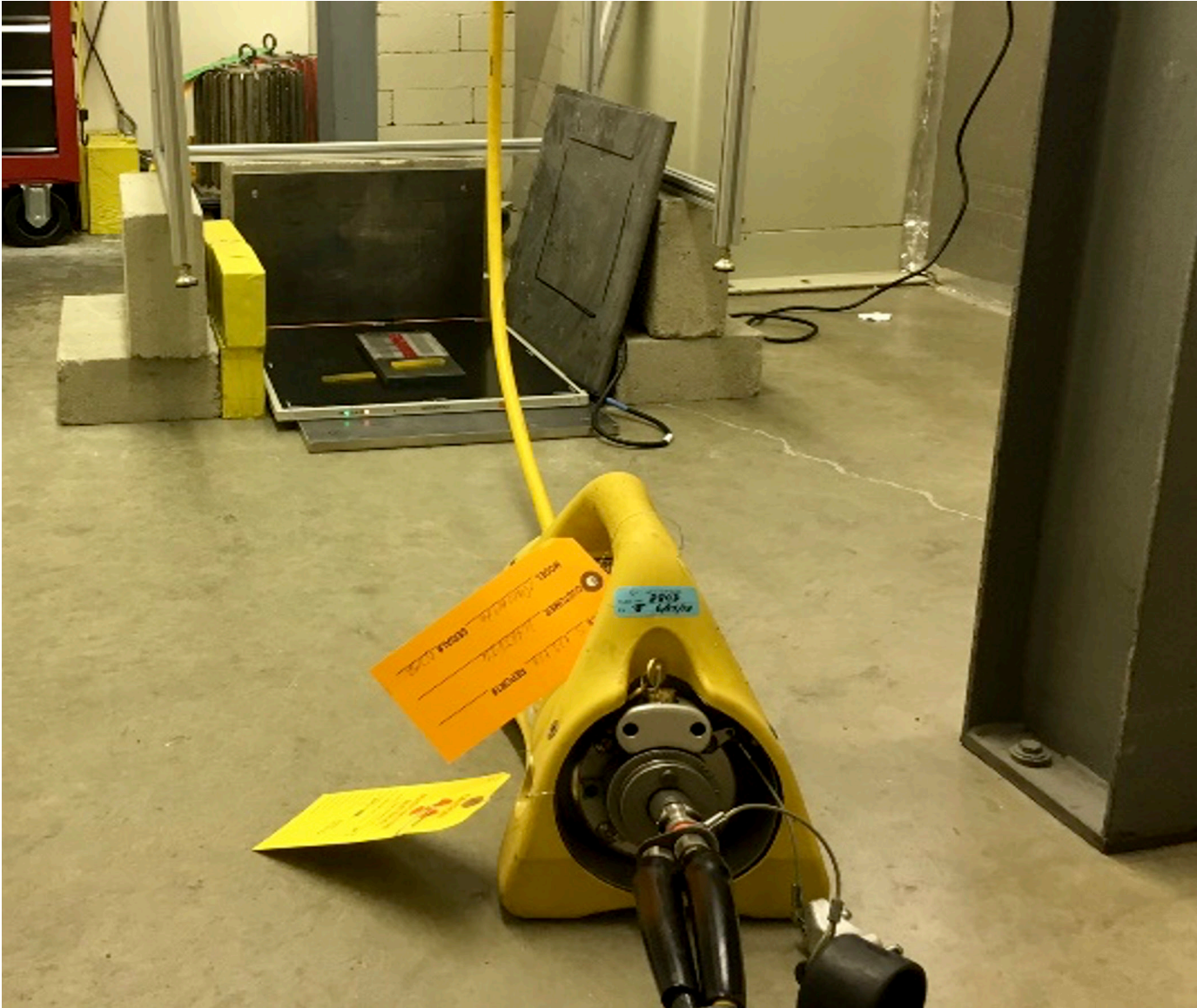
Figure 1: Experimental setup for 1/2-inch steel plate with a 139 mm pixel pitch HPX-DR DDA, as described in [13] and [14]
