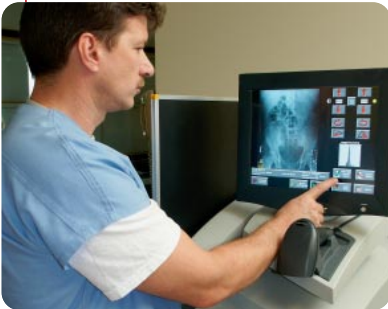
Student technologist Robert Richardson reviews an image on the Kodak DirectView CR 850 computed radiography system. The Kodak CR 850 system offers a throughput of up to 104 cassettes an hour.
