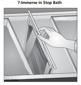
When the timer ends, place the film in the stop bath for 30 seconds. Agitating moderately, lift from the stop bath and drain well.
