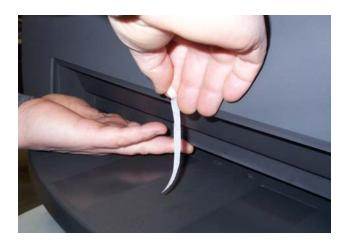
If neither of these tests confirm airflow, then it's probably a good time to change the foam (P/N 2G3232) and filter (P/N 2G3224). The replacement procedure is very simple... just pull out the dirty ones and insert the new ones:
