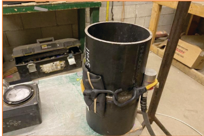
Figure 5: Film MX125 installed in 6" pipe test coupon, double-side single-view technique, from White [2]
