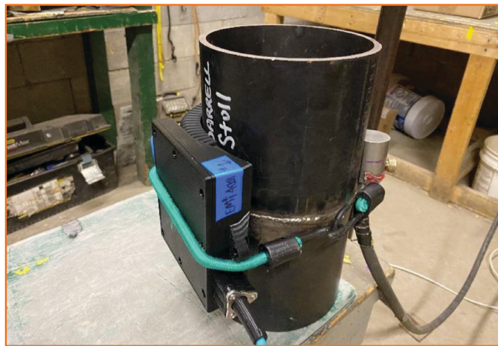
Figure 3: Conformable DR detector installed in 6" pipe test coupon, double-side single-view technique, from White [2]
