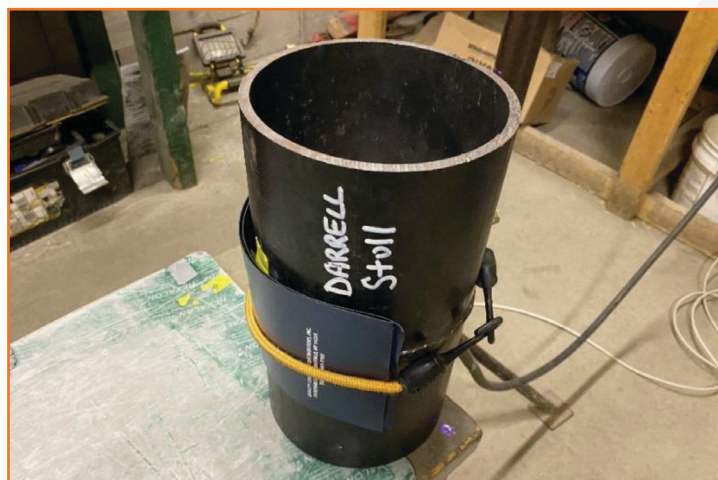
Figure 4: HPX-1+ HR imaging plate installed in 6" pipe test coupon, double-side single-view technique, from White [2]
