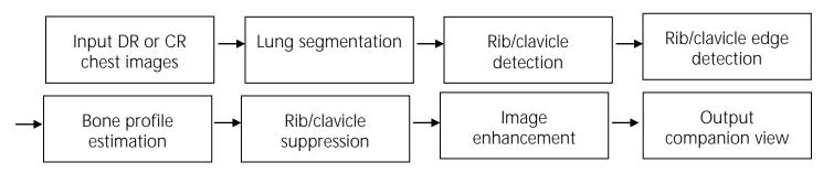
Figure 1: Image-processing chain to generate a bone-suppressed companion view
