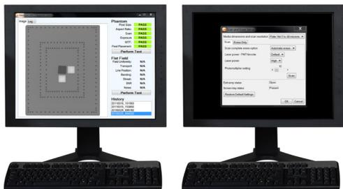
**System Status – Diagnostic Tool** – optional accessory allows user to monitor system stability per ASTM E2445.
