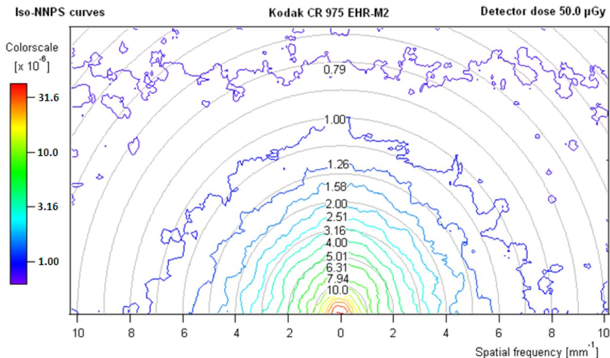
Figure C2: Iso-frequency and iso-NNPS curves of the Kodak CR 975 EHR-M2 system at 50  $\mu\text{Gy}$  (RQA-M2)
