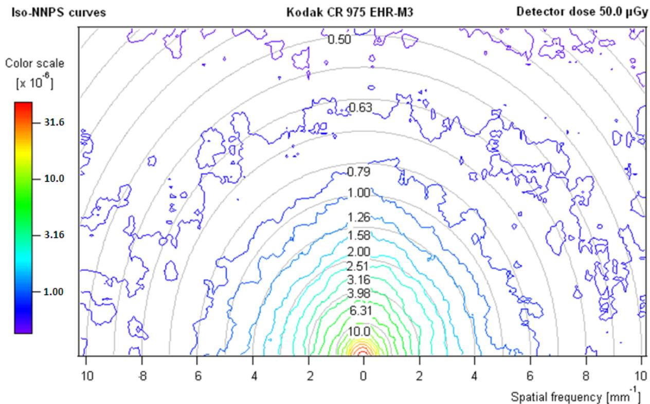
Figure C3: Iso-frequency and iso-NNPS curves of the Kodak CR 975 EHR-M3 system at 50  $\mu\text{Gy}$  (RQA-M2)
