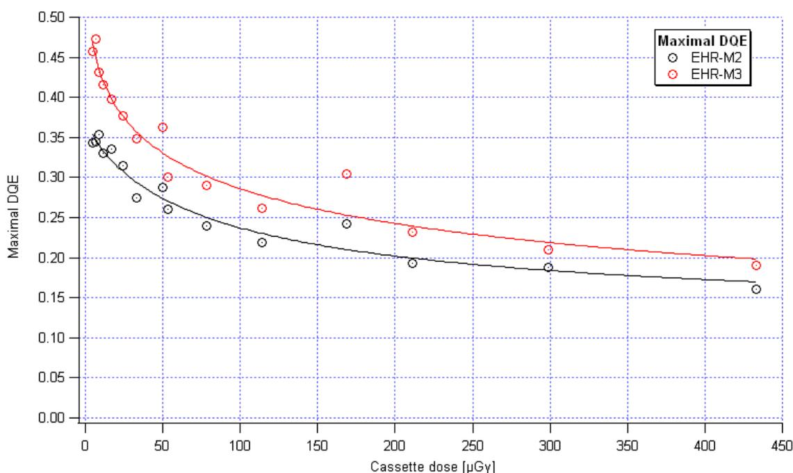
Figure E2: Maximal (low-frequency) DQE of the Kodak CR 975 EHR-M2 and EHR-M3 cassettes (RQA-M2)
