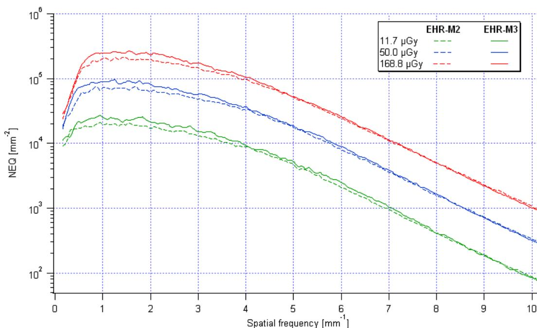
Figure D1: NEQ of the Kodak EHR-M2 and EHR-M3 cassettes at three doses
