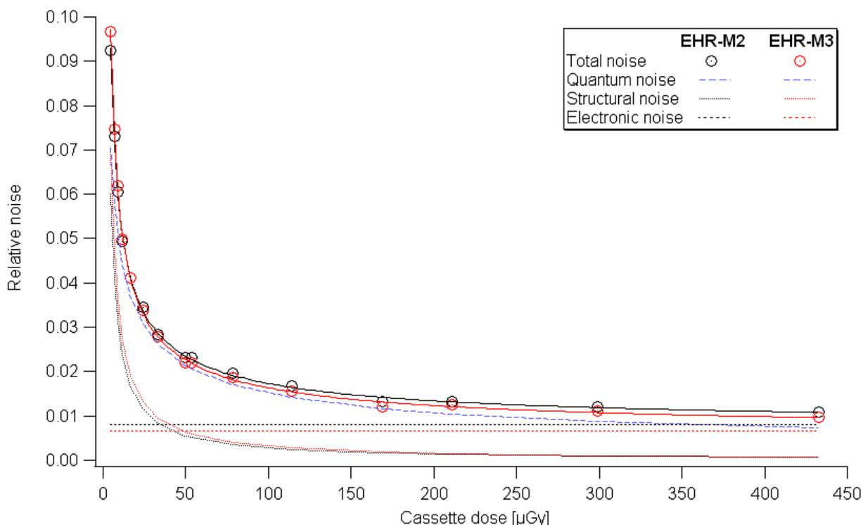
Figure C4: Relative noise of the Kodak CR 975 EHR-M2 and EHR-M3 cassettes (RQA-M2)
