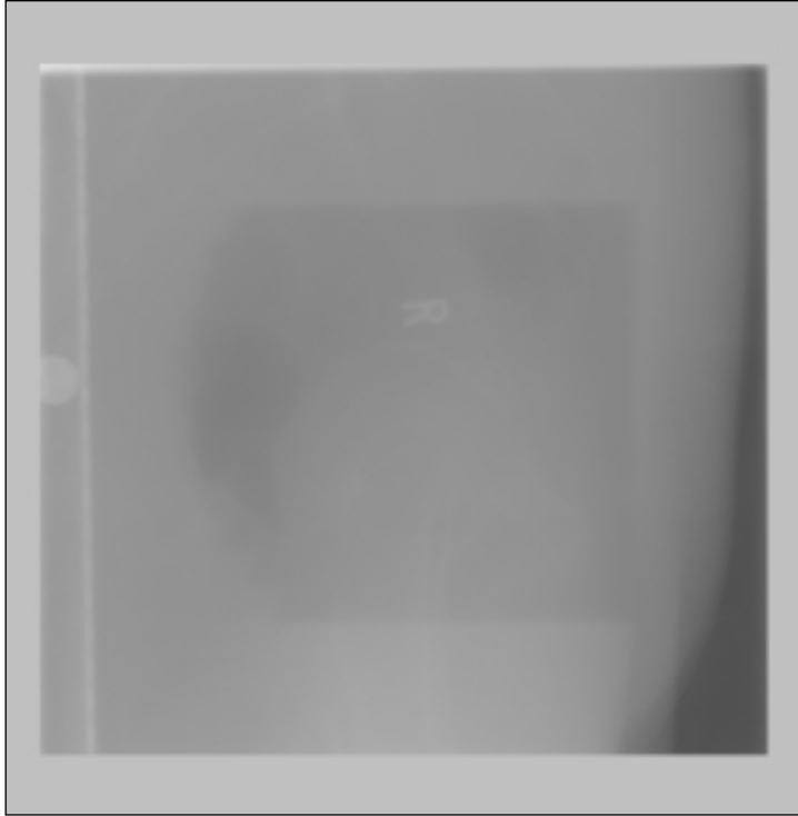
Figure 7. The solid gray area outside the collimation shows that the image processing algorithms have correctly identified the unexposed areas of the image. The image analysis is only based on the localization exposure and not scattered or background signals.
